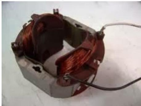
Gambar 2.6 stator motor universal
