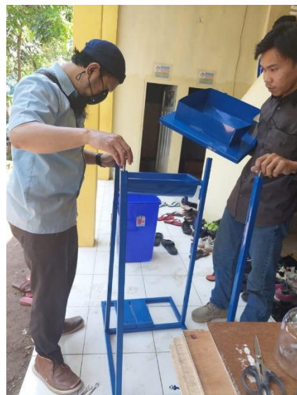
Gambar 4. Perakitan Alat cuci tangan Portabel Sistem Knockdown
