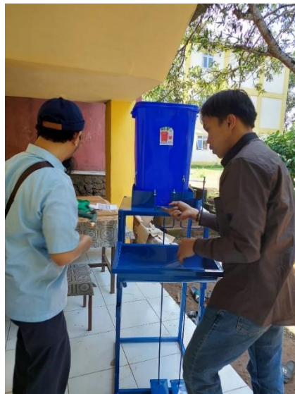
Gambar 4. Perakitan Alat cuci tangan Portabel Sistem Knockdown
