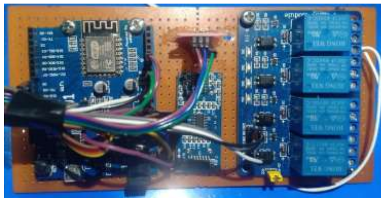
Fig. 6. Installation of the HC-SR04 ultrasonic sensor and water level sensor on the Wemos D1 board ESP8266 module
