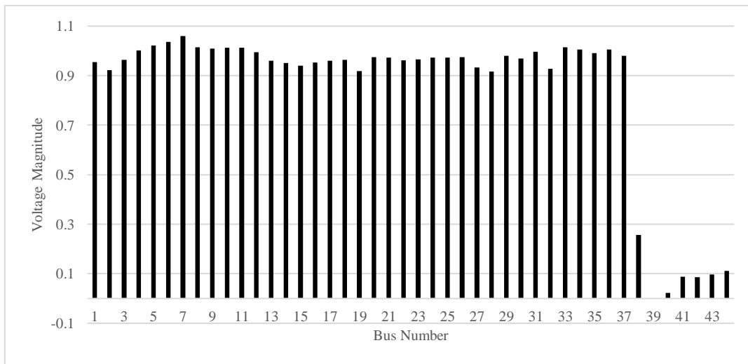
Fig. 6. Curves of The Bus Voltage Magnitude Per Unit Fault at Palopo Bus Using The New FFA-ABC Hybrid Method
