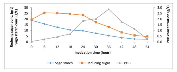
Figure 1. Process of bioconversion of sago starch to PHB by B.megaterium PSA10 during cultivation
