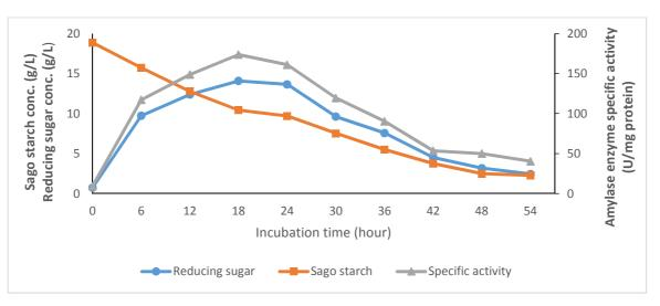
Figure 2. Process of sago starch hydrolysis by *B. megaterium* PSA10 and reducing sugar concentration formed on sago starch minimal media during cultivation
