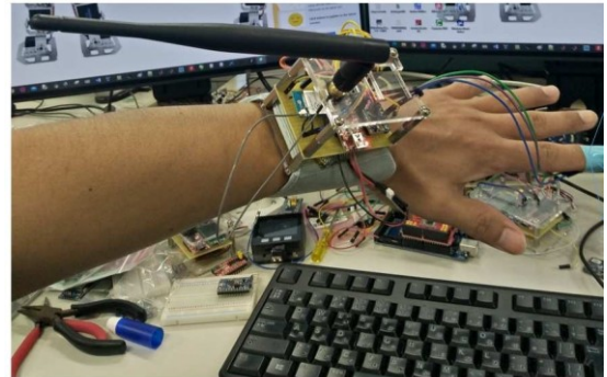
Fig.5. Fingertip Pulse sensor position
