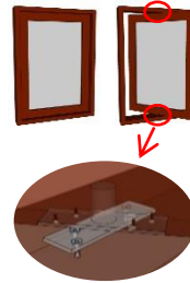
Gambar 4.20 : Detail jendela pivot Sketch : Andi Abidah, Muh. Idhil Maming
