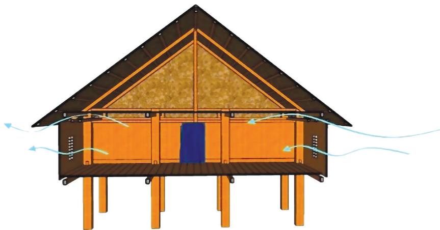
Figure 9. Cross ventilation (sketch: Andi Abidah 2020).
