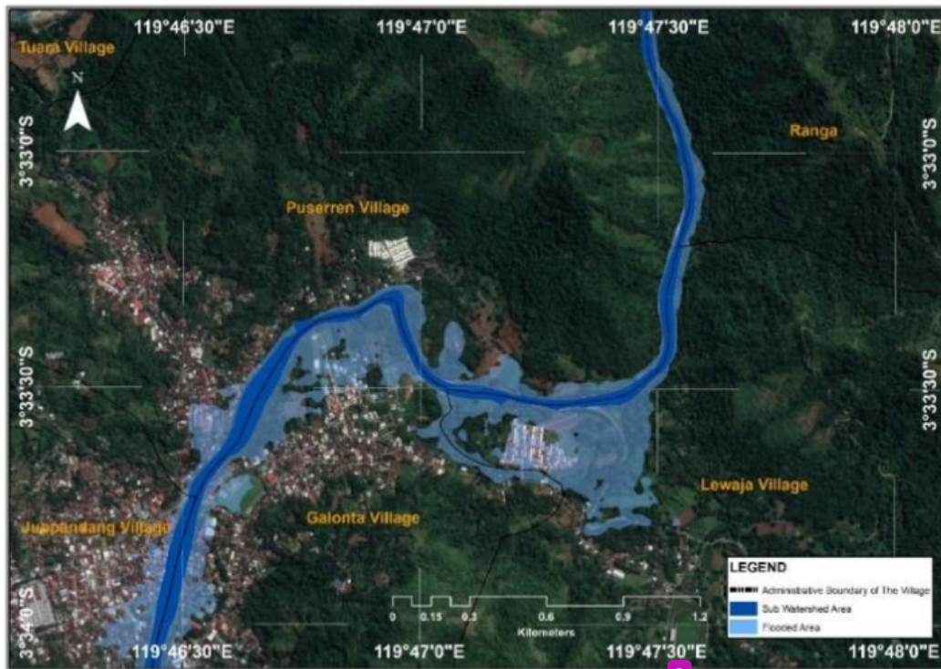
Fig. 6. Flood inundation distribution map of the Mata Allo Sub-watershed at the Q100 year return period.
