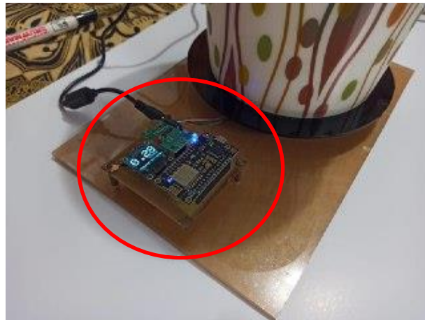
Figure 6. Automatic Waste Weighing Tool using Digital Scales
