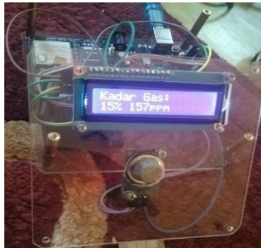
Figure 4. MQ6 gas sensor testing
