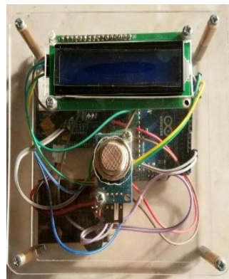
Figure 3. Front display of Gas leakage detection tool
