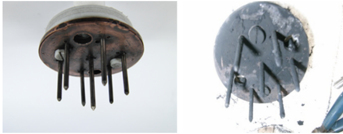
Fig. 7.2 Condition of antennas/electrodes before and after methane hydrate decomposition
