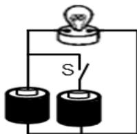
In the circuit below, the two batteries are identical and ideal (no internal resistance). The electric current in the circuit when switch S is disconnected is I
