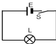
The circuit below consists of a battery E, lamp L, switch S and conductor wire
