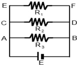
The picture on the right shows a battery in parallel with three different resistances
