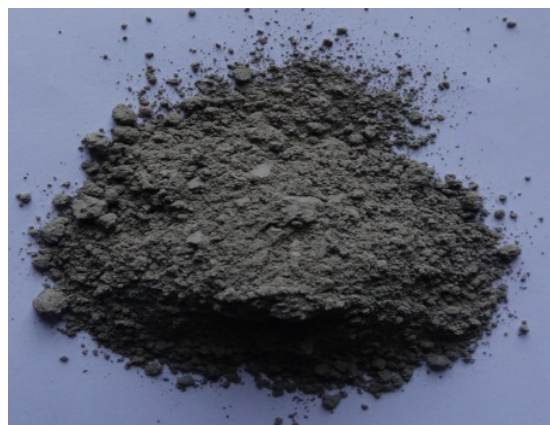
Figure 1. Sample of furnace nickel slag powder.
