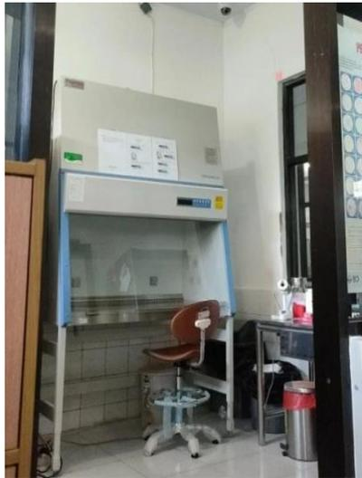
Gambar 6. 34. *Laminar Air Flow*
