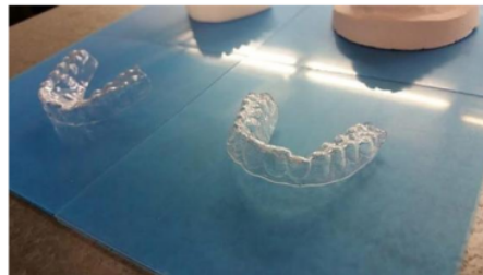
Fig. 7. Molding results using vacuum forming with PET plastic material
