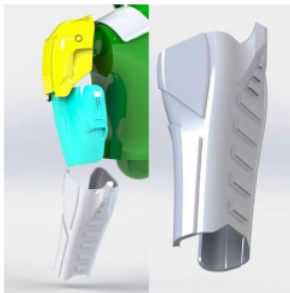
Fig. 4. The 3-Dimensional digital visual presentation of products that will be created using a vacuum forming
