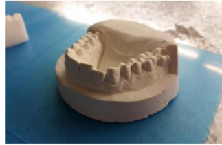
Fig. 6. The pattern is made to be used as a mold base in the vacuum forming process. This mold is made using a 3D printer machine
