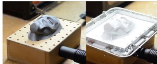
Fig. 8. Using a vacuum forming device is possible to produce large quantities
