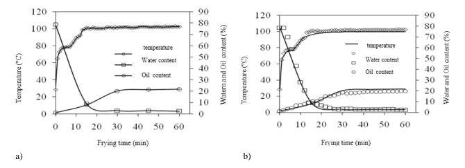
Figure 5: History temperature, moisture reduction and oil absorption simultaneously in jackfruit solids during the frying process at the oil temperature of  $100^{\circ}$ C with the vacuum pressure of 90 kPa; a) observational data; and b) the results of simulation models.
