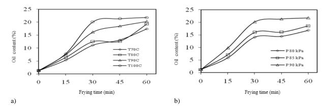
Figure 4: Increased levels of oil in jackfruit solids; a) temperature variation in the vacuum pressure of 90 kPa; and b) vacuum pressure variation in the oil temperature of  $100^{\circ}$ C.
