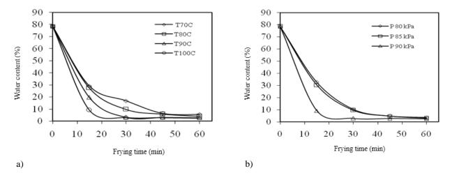
Figure 3: Decrease of the water content of jackfruit solids during frying; a) temperature variation in the vacuum pressure of 90 kPa; and b) vacuum pressure variation in the oil temperature of 100<sup>o</sup>C.
