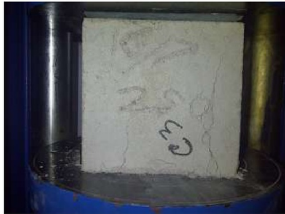
Fig. 1. Testing of concrete compressive strength with sample of cube
