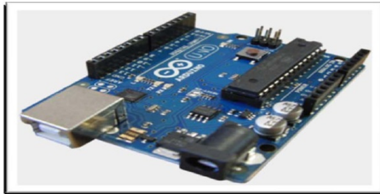
Fig. 4: Kit arduino as an interface of microcontroller
