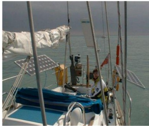
Figure 12 – Solar cell energy at fisherman vessel
